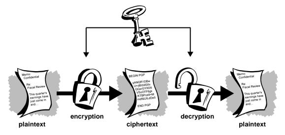
Figure 1-2. Conventional encryption
