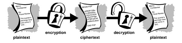
Figure 1-1. Encryption and decryption
